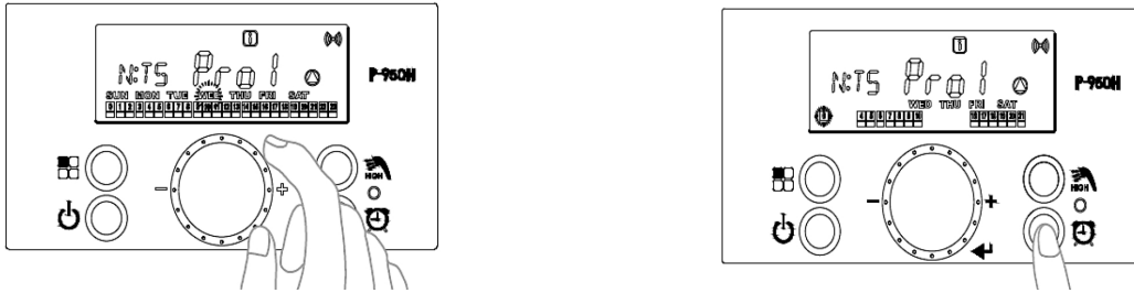
Figure 60 - A - Selecting the Day, Turning the Dial to Other Days, B - Setting the Time
