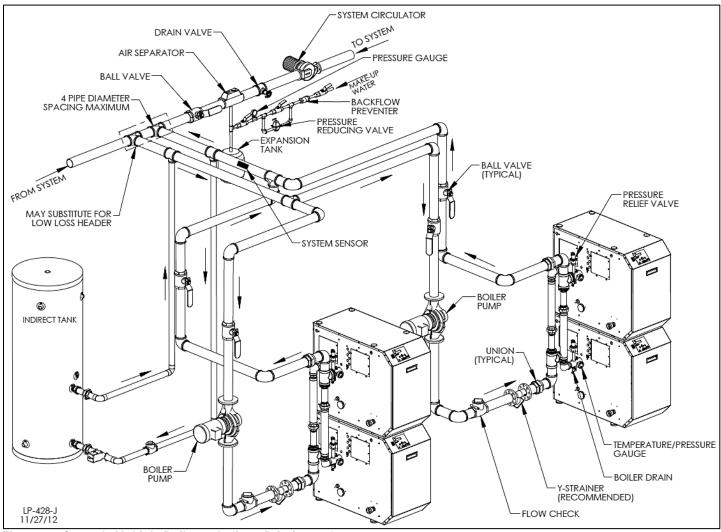
Figure 8 - Cascade Multiple Boilers - Indirect Priority on One
