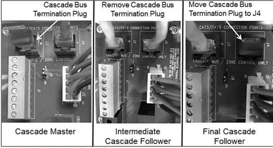
Figure 25 - Cascade Resistor Plug Installation Detail
