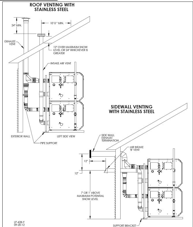
Figure 14 - Sidewall Venting with Stainless Steel
