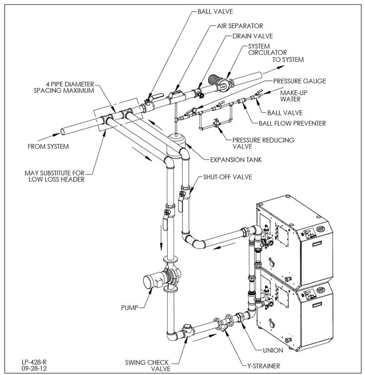
Figure 9 - Single Boiler Space Heating
