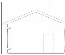
Figure 16 - Combustion Air From Outdoors
