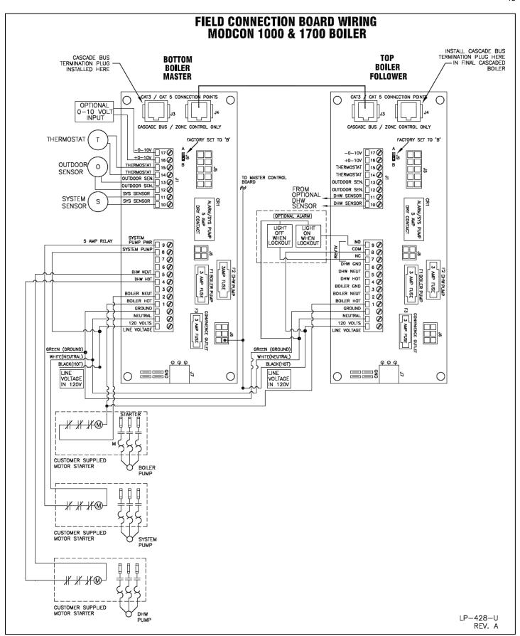
Figure 26 - Mod Con Cascade Master and Follower Wiring
