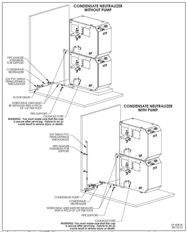
Figure 12 – Condensate Piping NOTE: Blow water into the condensate collector to remove any foreign matter that may block the line.
