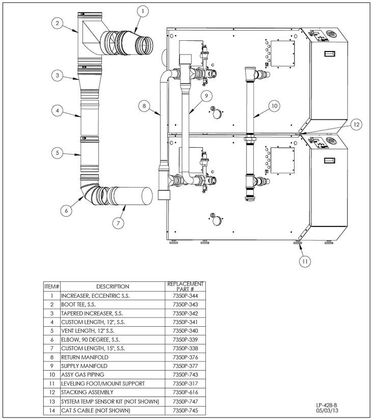
Figure 31 - MOD CON 1700 External Parts Blowout
