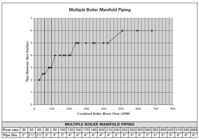
Figure 6 - Multiple Boiler Manifold Piping
