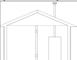
Figure 18 - Combustion Air From Indoors
