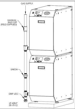
Figure 20 - Gas Connection Detail
