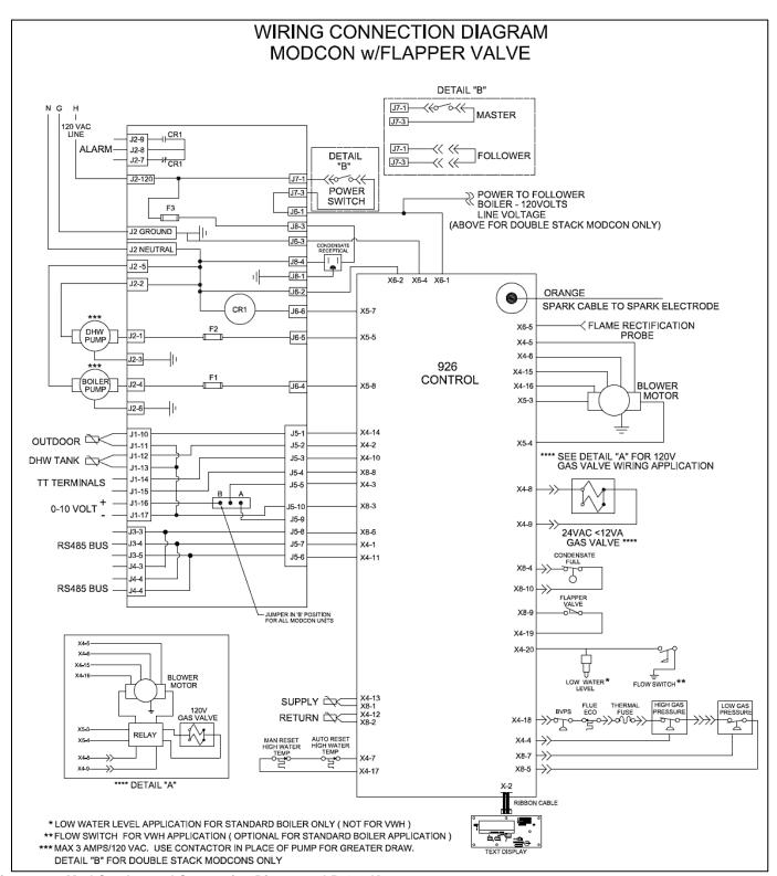
Figure 27 - Mod Con Internal Connection Diagram - LP-428-K
