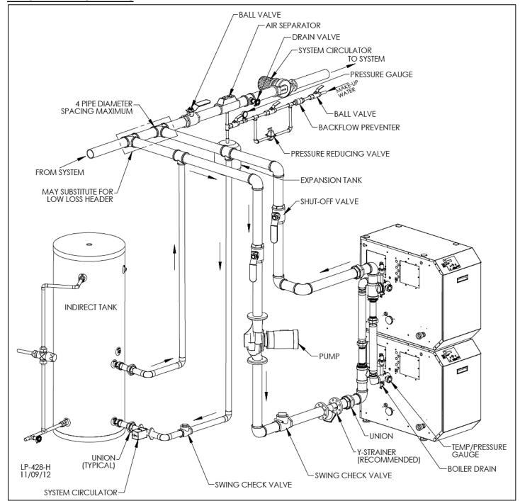
Figure 7 - Single Boiler Space Heating - Indirect Priority
