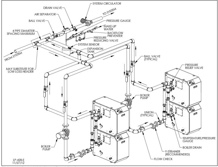
Figure 10 - Cascaded Boilers - Space Heating
