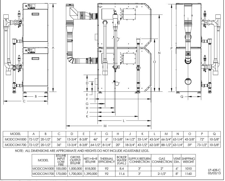
Figure 2 - Specifications and Dimensions
