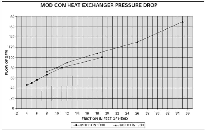
Figure 5 - Heat Exchanger Pressure Drop Chart
