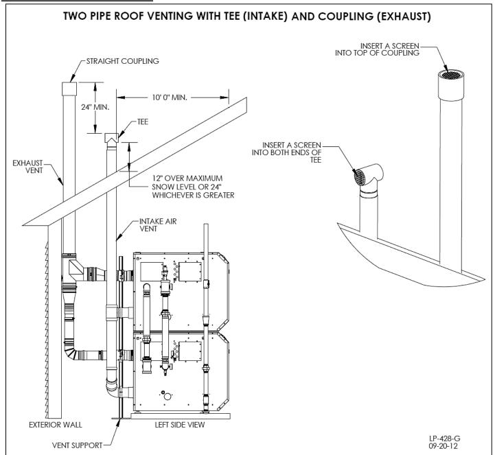
Figure 15 - Two Pipe Roof Venting with Tee and Coupling
