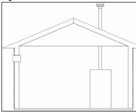
Figure 19 - Combustion Air From Outdoors - Single Opening
