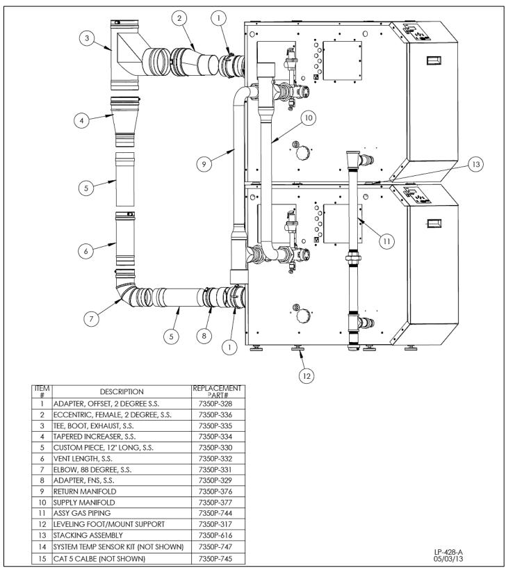
Figure 30 - MOD CON 1000 External Parts Blowout
