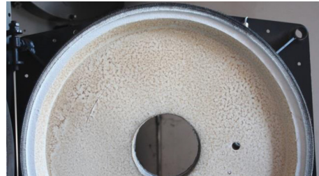
Figure 40 - Combustion Chamber Door With Installed Seal
