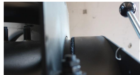
Figure 41 - Closed Door with Properly Fitted Seal
