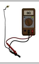
② ► Connect multimeter leads to the Water Outlet Sensor socket and measure the resistance value (If value is  $0\Omega$  it's a sensor's malfunction so replace it)
