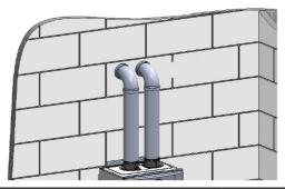
$\ensuremath{\,^{\circlearrowleft}}$  Please check tthe blockage of flue (intake and exhaust pipes)
