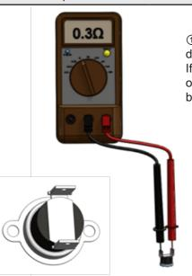
① Check burner plate for distortion or burn marks. If plate shows signs of overheating, replace entire burner plate assembly.
