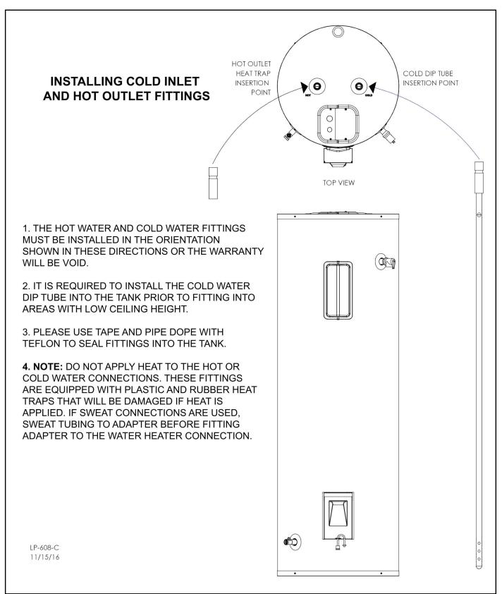
Figure 3 - Installing Cold Inlet and Hot Outlet Fittings
