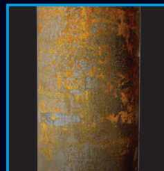
Top Competitor's Glass-lined Tank Very Heavy
