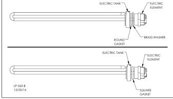
Figure 7 - Heating Element Detail
