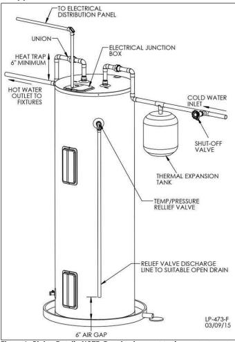
Figure 4 - Piping Detail - NOTE: Drawing is meant to demonstrate system piping concept. Heat traps are optional.
