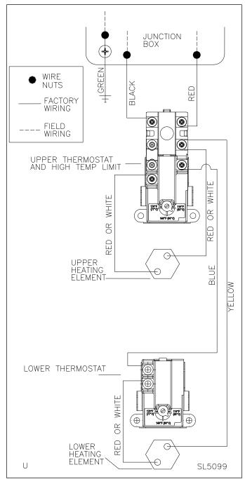
Figure 6 - Dual Element Model Wiring Detail, Non-Simultaneous Element Operation - Green Wire for Grounding the Water Heater
