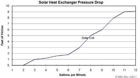
Figure 14 - Pressure Drop through the Solar Heat Exchanger
