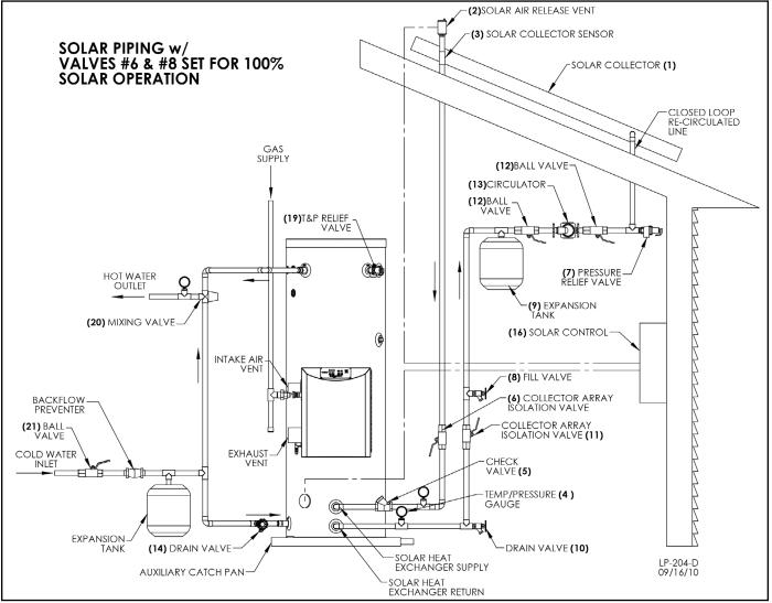
Figure 9 - Potable Water Piping Application. Meant to demonstrate piping concept only. Installer is responsible for all equipment and detailing per local codes.
