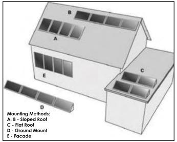
Figure 1 - Suggested Solar Collector Mounting Designs
