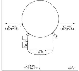
Figure 4 - 160 and 199kBTU Model Service Clearances
