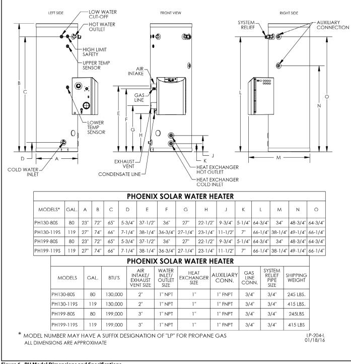
Figure 6 - PH Model Dimensions and Specifications
