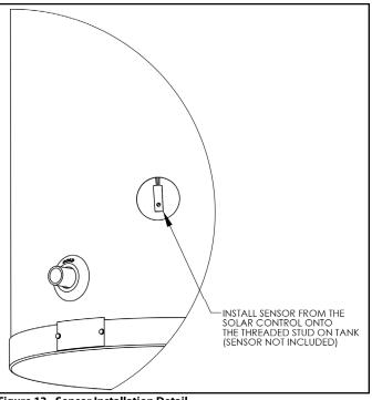
Figure 13 - Sensor Installation Detail
