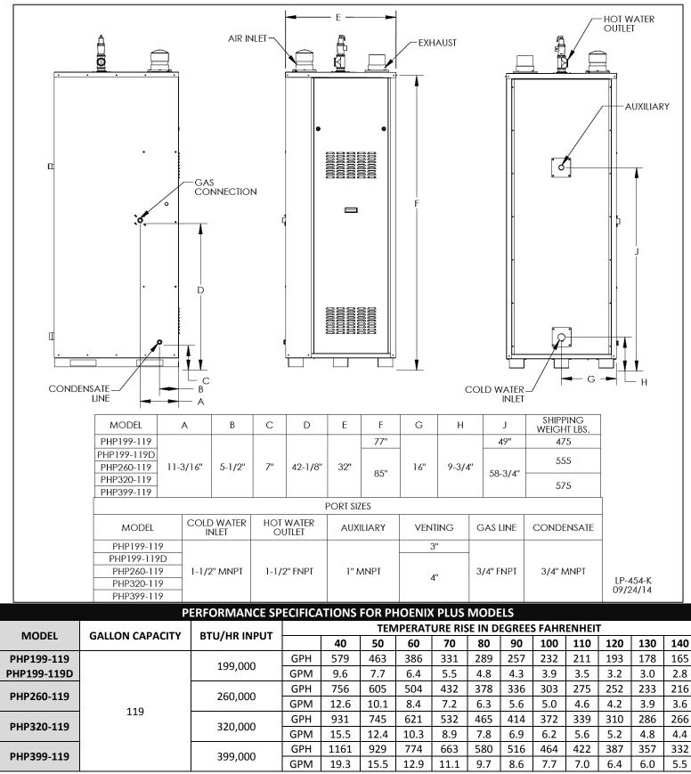
Phoenix Plus Performance – 95% Thermal Efficiency Used for Calculations
