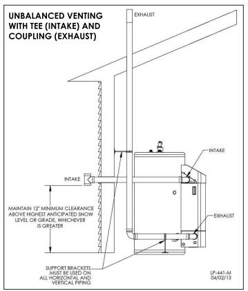
Figure 11 - Unbalanced Venting - Roof Exhaust and Sidewall Intake
