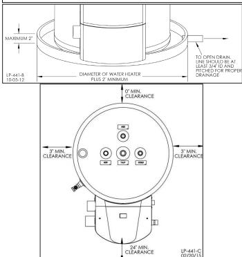
Figure 1 - Drain Pan Dimensions and Recommended Service Clearances
