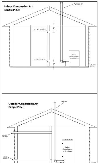
Figure 14 - Indoor and Outdoor Combustion Air - Single Pipe
