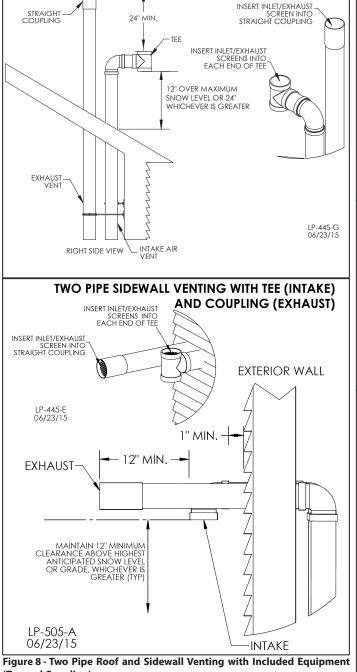
TWO PIPE ROOF VENTING WITH TEE (INTAKE)
