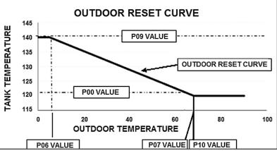
Figure 24 - Outdoor Reset Curve
