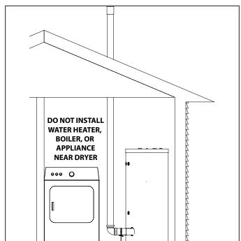
Figure 13 - Do Not Place Appliance Near Dryer
