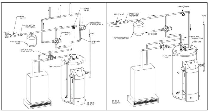
Figure 5 - Piping with Air Handler on Side
