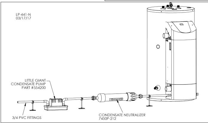
Figure 15 - Condensate Piping
