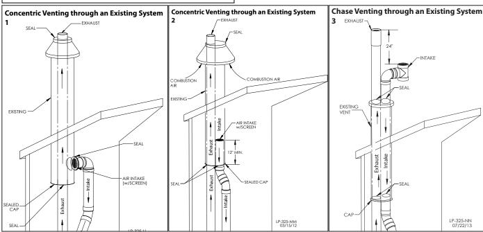
Figure 12 - 1, 2 - Concentric Venting Through an Existing System, 3, Chase Venting Through an Existing System
