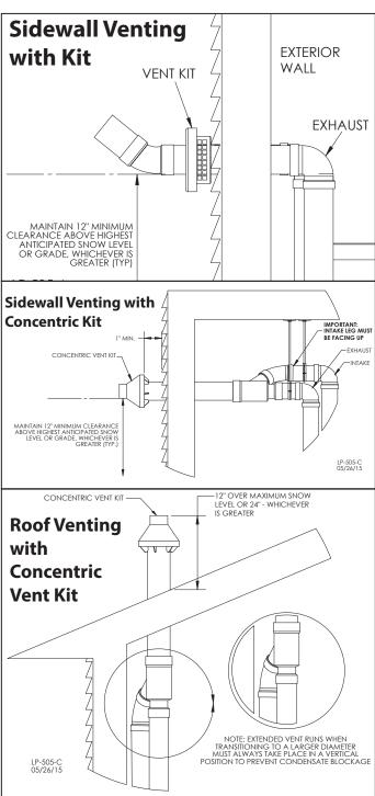
Figure 9 - Venting with Optional Kits (NOT INCLUDED WITH THE WATER
