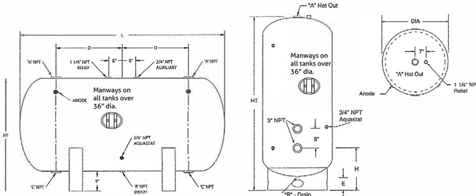
Horizontal tanks are shipped with saddles attached to the tank.
