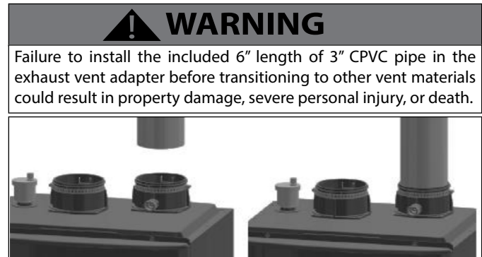
Figure 19 - Correct Installation into the Boiler Collar
